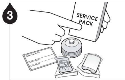
3 Check the grease pouch capacity and the service pack items (battery pack, grease pouch & dust cover).
