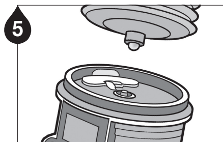
5 Purge the grease pouch until grease comes out of the tip.
